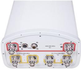
6-port sector antenna, 2x 698–896 and 4x 1695–2360 MHz, 65° HPBW, 2x RET. Both high bands share the same electrical tilt.
