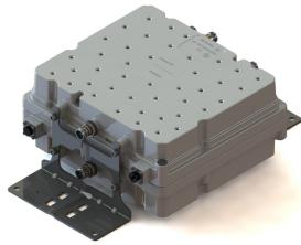
Dual Band Tower Mounted Amplifier, 700//850 MHz, 13 dB, 2 BTS & 2 ANT ports, AISG with 1 RET connector (2 devices with 2 sub-units), with 4.3-10 connectors
