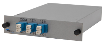
CWDM Fiber Optical Module, Demux, 1350-1410 nm, LC/PC, 4 channels
